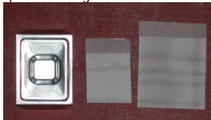
Manufactured from solvent resistant nylon bags that provide an excellent fluid exchange and maximum tissue safety during processing.
